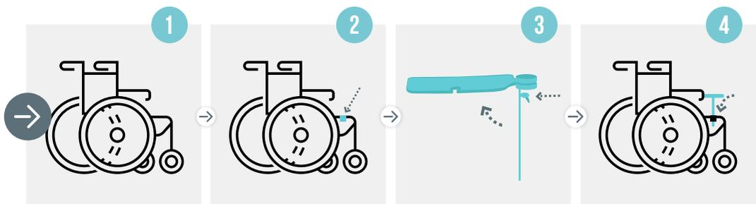
1 VOTRE FAUTEUIL ROULANT → 2 AJOUTER UNE FIXATION GLISSIÈRE → 3 DÉPLIER LA TABLETTE PUIS PIVOTER VERS L'INTÉRIEUR JUSQU'À LA BUTÉE → 4 INSÉRER LA TIGE DE LA TABLETTE DANS LA FIXATION GLISSIÈRE
